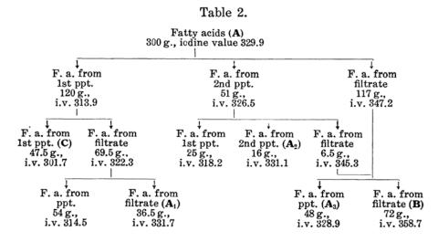
From their iodine values, the fatty acids fractions  $(A_1)$ ,  $(A_2)$  and  $(A_3)$  are considered to consist essentially of an acid  $C_{20}H_{32}O_2$ ; the fraction (B) contains a more highly unsaturated acid  $C_{20}H_{30}O_2$  in addition to the acid  $C_{20}H_{32}O_2$ , while the fraction (C) contains less unsaturated acids besides the acid  $C_{20}H_{32}O_2$ .
